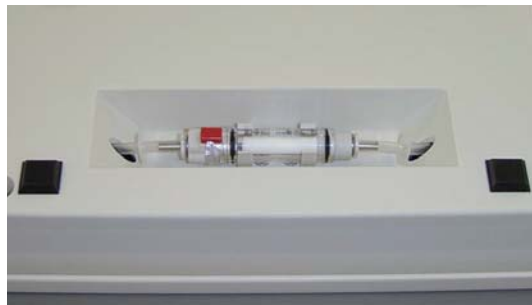
Air Filter Unit
